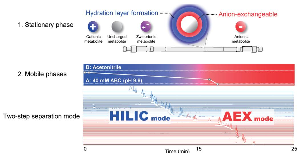
Fig. 1. Schematic of chromatographic separation and mass spectrometric detection of polar metabolites based on unified-HILIC/AEX/HRMS. ABC, ammonium bicarbonate; AEX, anion exchange; HILIC, hydrophilic interaction liquid chromatography; Unified-HILIC/AEX/HRMS, unified-hydrophilic interaction/anion exchange liquid chromatography/high-resolution mass spectrometry.
