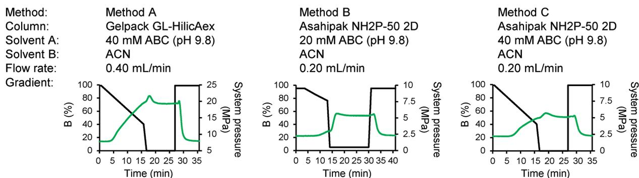
Fig. 2. Comparison of differences in specific parameters for each of the LC analysis conditions. ABC, ammonium bicarbonate; ACN, acetonitrile; LC, liquid chromatography.
