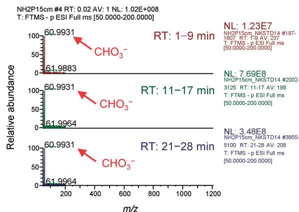
Fig. 6. Monitoring and comparison of bicarbonate ions in three LC/HRMS methods. BPCs, EICs of bicarbonate ions, and average mass spectra in the  $m/z$  50–200 at each RT for negative ionization for methods A (A), B (B), and C (C). BPCs, base peak chromatograms; EICs, extracted ion chromatograms; HRMS, high-resolution mass spectrometry; LC, liquid chromatography; RT, retention time.
