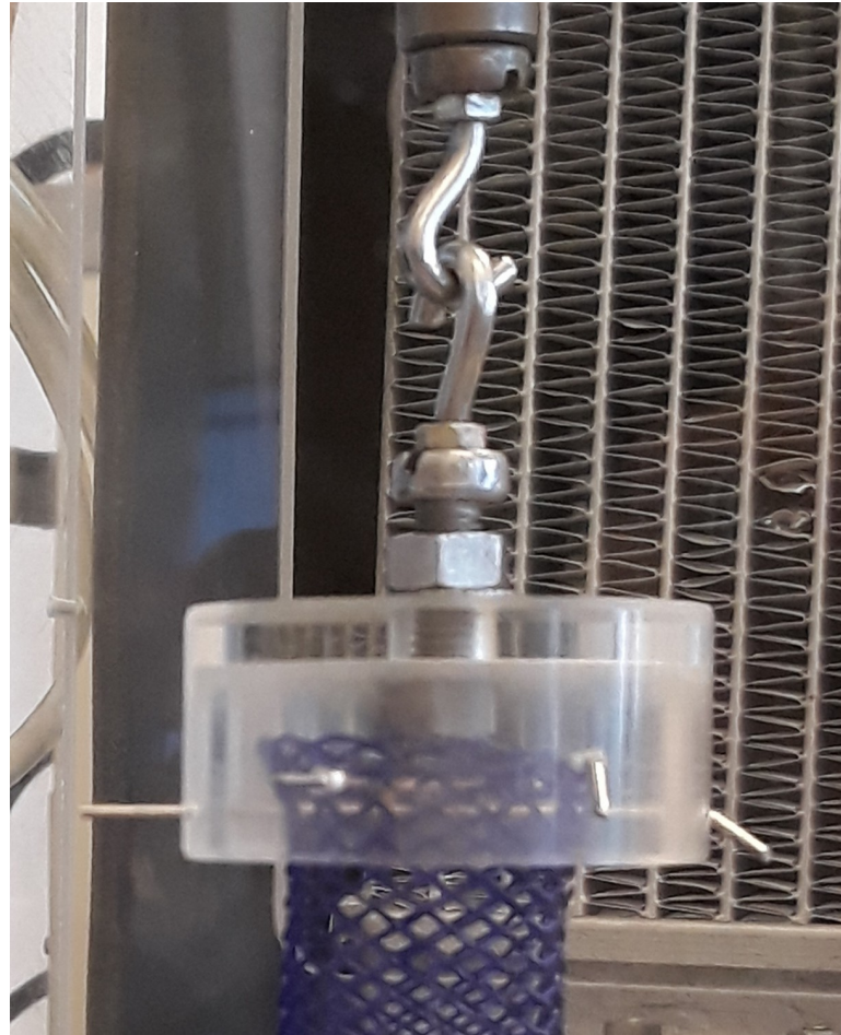
Fig 3. Details of the custom holding tool. The tool consists of a hollow cylinder with one open end and one closed end. A hook is mounted to the closed end, allowing its attachment to the measuring device. There are three small holes in the cylinder shell for the transverse attachment of stainless-steel needles.
