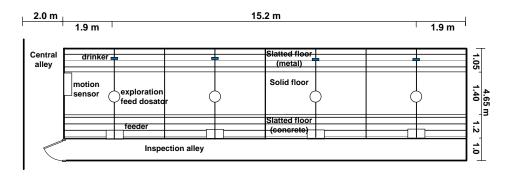
Figure 1. Layout of one of the nine rooms with eight pens with motion sensors and dosators.
