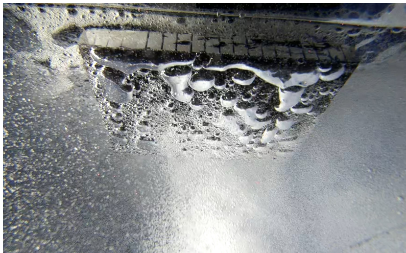
Figure 10 The small (1 mm) bubbles from the diffusers were observed joining and forming much larger bubbles on acrylic and fouling release panels (200 × 150 mm) fixed in a horizontal orientation. If this could be maintained, it could potentially be exploited to create a barrier between larvae and static coastal infrastructure.
