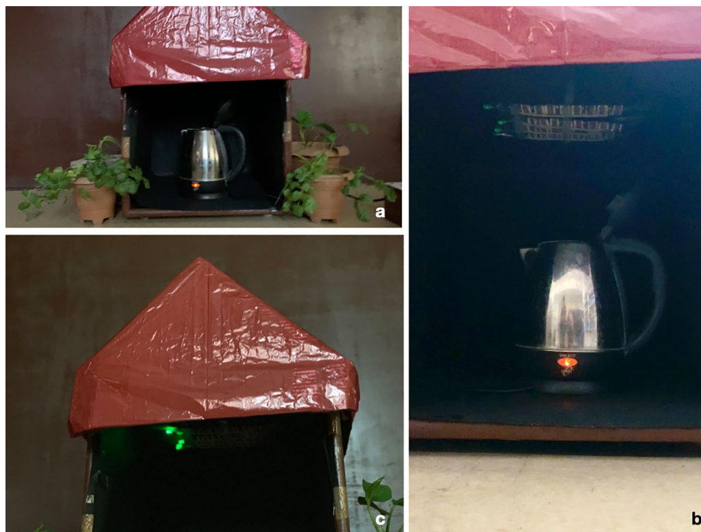
Figure 8. The water-vapor panels for futuristic homes. (a) The set-up shows the prototype of a model home with the panels made up of 'brine-silk cocoon protein bio-battery.' (b) The panels receive water vapor from the bottom. The glowing devices as seen on the roof. (c) The brightly glowing devices on the roof of the model house.
