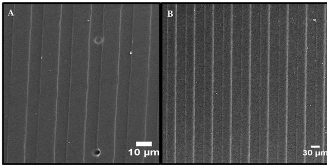
**Figure 1** Scanning electron microscopy images of micropatterned films. (A) 10/10  $\mu\text{m}$  film, scale bar: 10  $\mu\text{m}$ , 1000 $\times$  magnification. (B) 30/30  $\mu\text{m}$  film, scale bar: 30  $\mu\text{m}$ , 200 $\times$  magnification.
