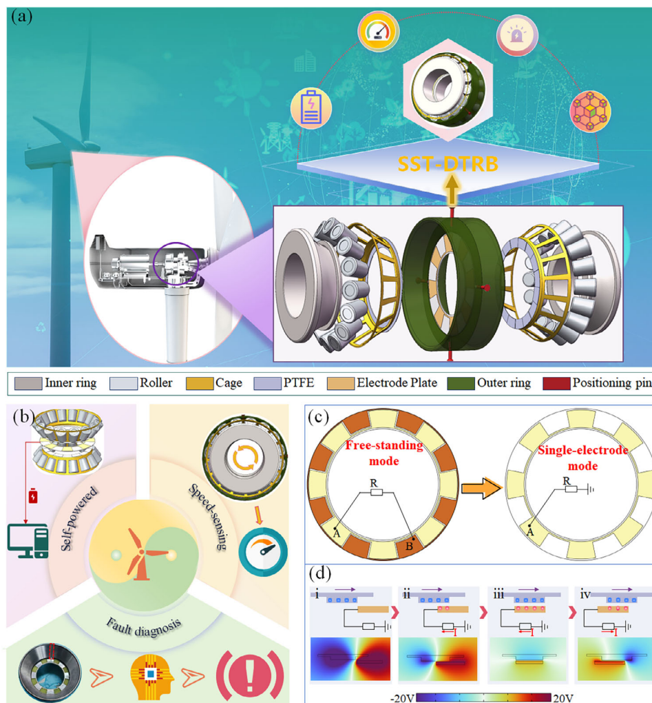
Figure 1. Application diagram and architecture of SST-DTRB: a) application diagram and structure, b) key advantages, c) comparison between free-standing layer mode and single-electrode mode, d) working principle of SST-DTRB.
