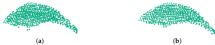
Figure 6. Comparison the original point cloud and moving least squares (MLS) processed point cloud. (a) Picking a leaf's point cloud from the whole point cloud. (b) Smoothing these point clouds with MLS method.
