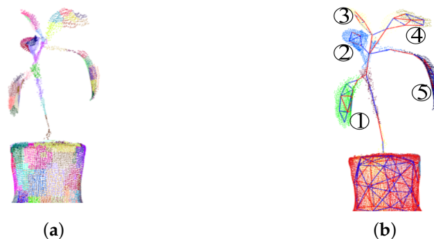
Figure 7. Segmentation leaves and stem with locally convex connected patches method (LCCP) algorithm. (a) Segmentation plant's point cloud into small regions. (b) Small regions into larger objects by convexity-concavity relationship.
