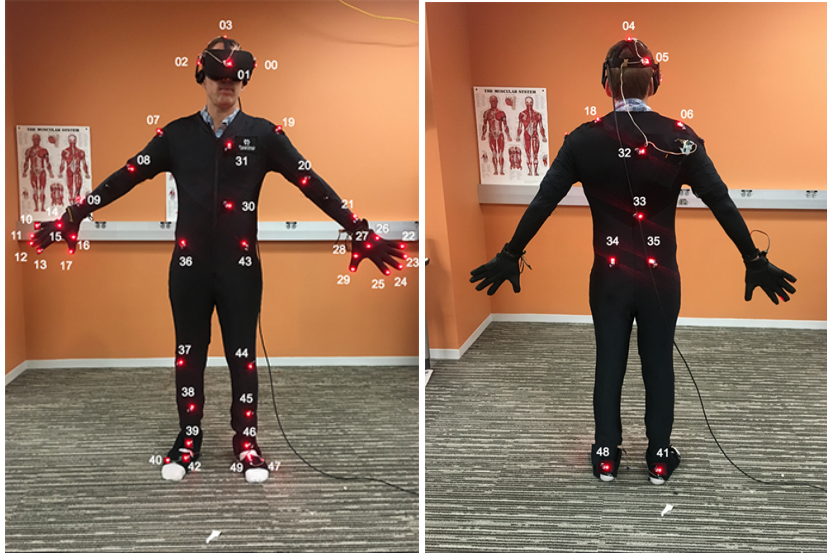
Figure S3: PhaseSpace suit with 50 active-pulse LED markers. The numbers next to the LED markers are the marker indexes used for recording the motion capture data. Related to Figure 2.
