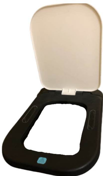
Figure 1. Prototype of the toilet seat, highlighting the electrodes' positioning.
