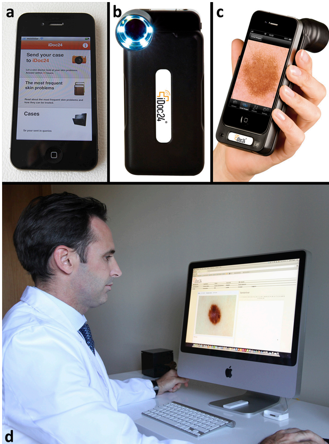
Figure 1. Technologic equipment used in the mobile teledermoscopy solution: (A) the smartphone (iPhone 4 ® ) with the iDoc24 ® app showing on the display; (B) the dermoscope (Fotofinder Handyscope ® ) with its six light-emitting diodes lit; (C) the dermoscope attached to the smartphone displaying a dermoscopic image of a reticular nevus; and (D) a dermatologist viewing a case on the Internet platform (Tele-Dermis ® ). [Copyright: ©2013 Börve et al.]
