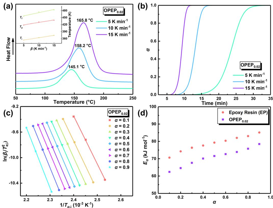
Fig. 2 (a) DSC curves of OPEP<sub>0.02</sub> sample in different heating rates; (b) relationship between conversion rate ( $\alpha$ ) and time; (c) linear fitting curves of  $\ln(\beta_i/T_{\alpha,i}^2)$  and  $1/T_{\alpha,i}$ ; (d) relationship between activation energy ( $E_\alpha$ ) and conversion rate ( $\alpha$ ).
