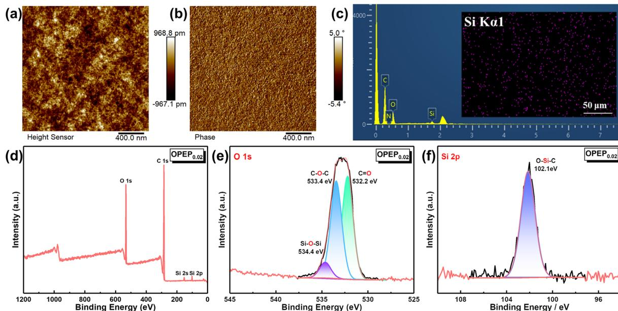
Fig. 6 (a and b) The surface morphology and phase diagrams of OPEP<sub>0.02</sub> sample; (c) the EDS mapping of OPEP<sub>0.02</sub> sample; (d–f) the XPS spectrum of OPEP<sub>0.02</sub> sample.
