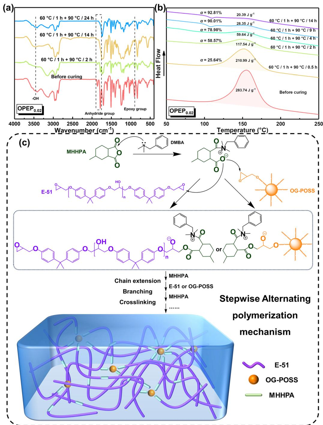
Fig. 4 (a) The on-line FTIR spectra of OPEP<sub>0.02</sub> sample; (b) the on-line DSC curve of OPEP<sub>0.02</sub> sample; (c) curing mechanism diagram of OPEP.
