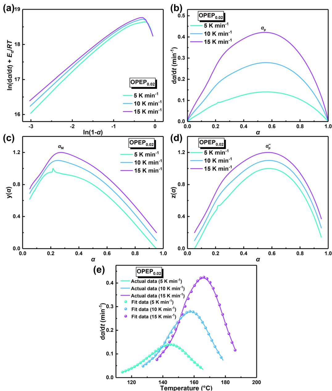
Fig. 3 (a) Relationship between  $\ln(d\alpha/dt) + E_a/RT$  and  $\ln(1 - \alpha)$ ; (b) relationship between reaction rate ( $d\alpha/dt$ ) and conversion rate ( $\alpha$ ); (c and d) normalized  $y(\alpha) \sim \alpha$  and normalized  $z(\alpha) \sim \alpha$  curves; (e) comparison of actual (lines) data and fit (dots) data: reaction rate ( $d\alpha/dt$ )  $\sim T$  curves.
