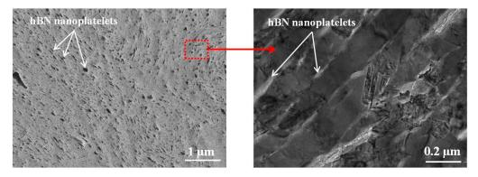
**Figure 4.** Microstructure of the composite particle after planetary ball milling recorded by transmission electron microscopy.
