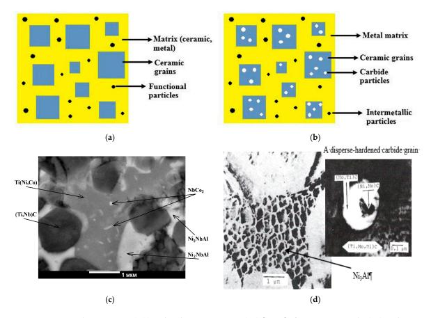
**Figure 2.** A schematic view (**a**,**b**) and real microstructures (**c**,**d**) [34,37] of ceramic materials: (**a**,**c**) with disperse-hardening binder; (**b**,**d**) with simultaneously reinforcing the grains and the binder.
