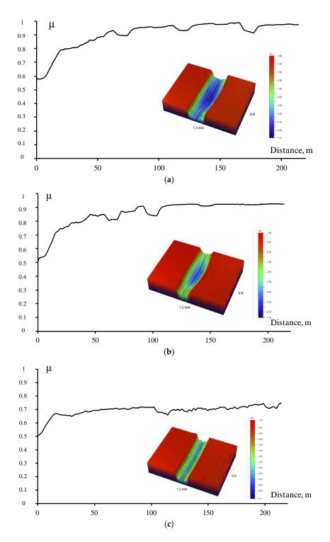
Figure 10. Results of tribological tests: (a) Fe–Ni–Mo; (b) Fe–Ni–Mo-CNT; (c) Fe–Ni–Mo-hBN samples.
