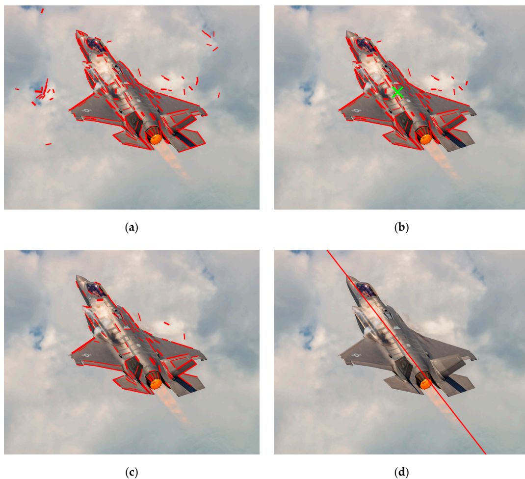
Figure 3. The results of line feature detection and fuselage extraction based on spatial, length and orientation consistency constraints: (a) line feature detection; (b) line clustering based on spatial consistency constraint; (c) length consistency constraint; (d) extraction of fuselage reference line based on parallel line clustering.
