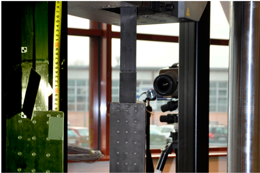
Figure 11. Recording the failure mode using the speed video camera with a high framing rate and an example of the view.
