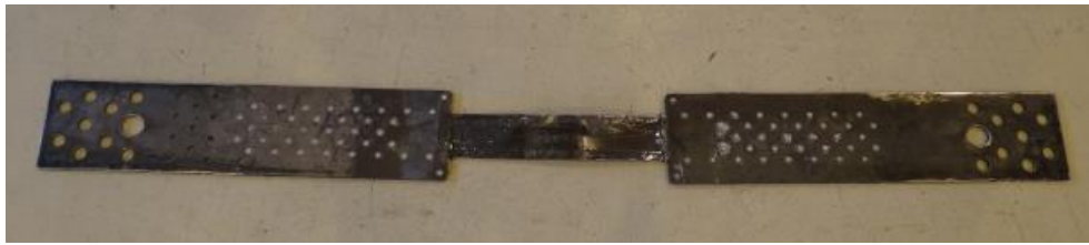
Figure 4. Double-sided N-type anchorage of the NPS I system tested in the S1N–S2N series.
