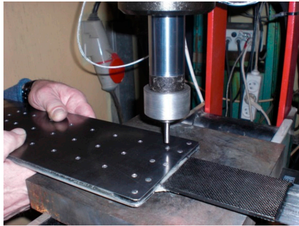
Figure 9. Rivet upsetting using the hydraulic press.
