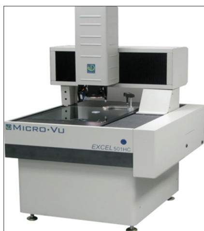
Figure 13: Micro-Vu: Excel gantry type visual measurement machine
