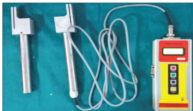
Figure 20: Transducer bite force measurement device with analog for bite equalization
