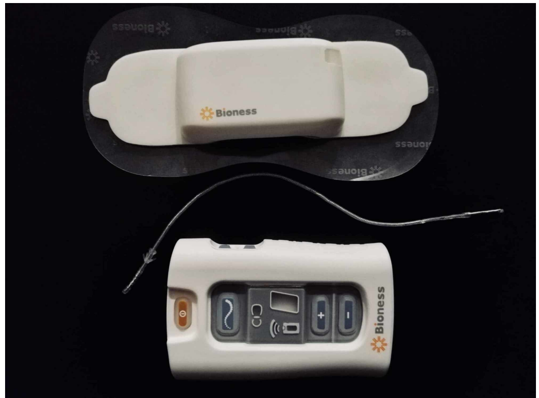
FIGURE 1: Image of a Percutaneous Peripheral Nerve Stimulator (Bioness StimRouter®, Valencia, CA), showcasing the three components of the system: the external pulse transmitter (EPT) and electrode patch, the implanted lead, and the patient programmer
