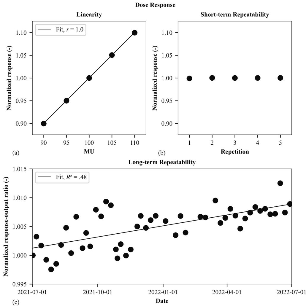
**Fig. 1.** Linearity of the megavoltage imager (MVI) response (a), short-term repeatability of the MVI response (b), and long-term repeatability of the MVI response (c) for beam output checks. The responses in (a) and (b) were normalized to the response for 100 MU and to the mean of the responses, respectively. The response-output ratios were normalized to the response-output ratio on July 1, 2021.
