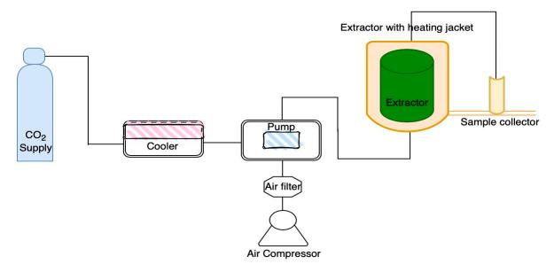
Figure 1. Overview of the SC-CO<sub>2</sub> system.
