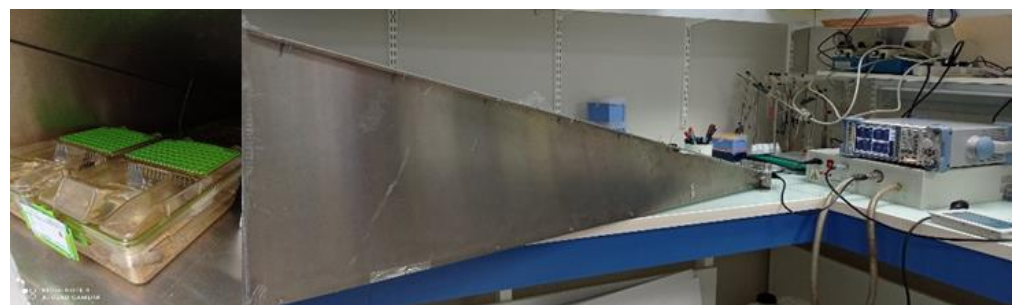
Figure 1. GTEM cell to explore in vivo studies.
