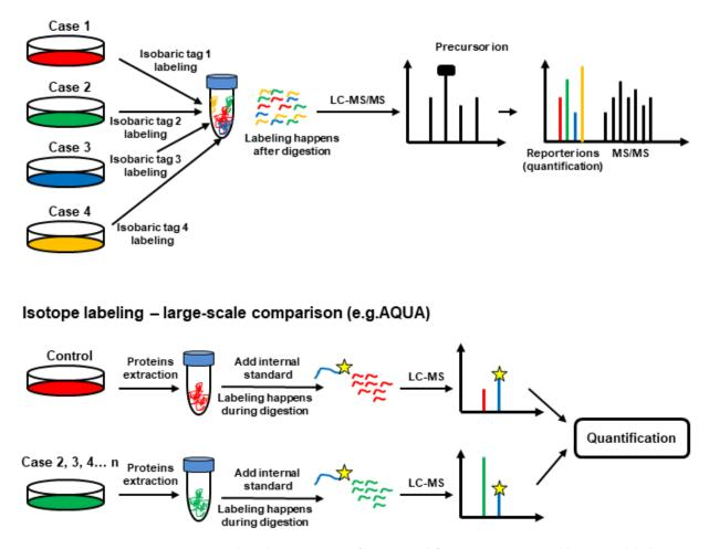
**Figure 4.** MS-based protein quantification workflow strategies via stable isotope labeling. Reprinted and adapted with permission from Woods, A.G.; Sokolowska, I.; Ngounou Wetie, A.G.; Channaveer-appa, D.; Dupree, E.J.; Jayathirtha, M.; Aslebagh, R.; Wormwood, K.L.; Darie, C.C. Mass Spectrometry for Proteomics-Based Investigation. *Adv. Exp. Med. Biol.* **2019**, *1140*, 1–26. [26]. Copyright @ 2019, Springer Nature Switzerland AG.
