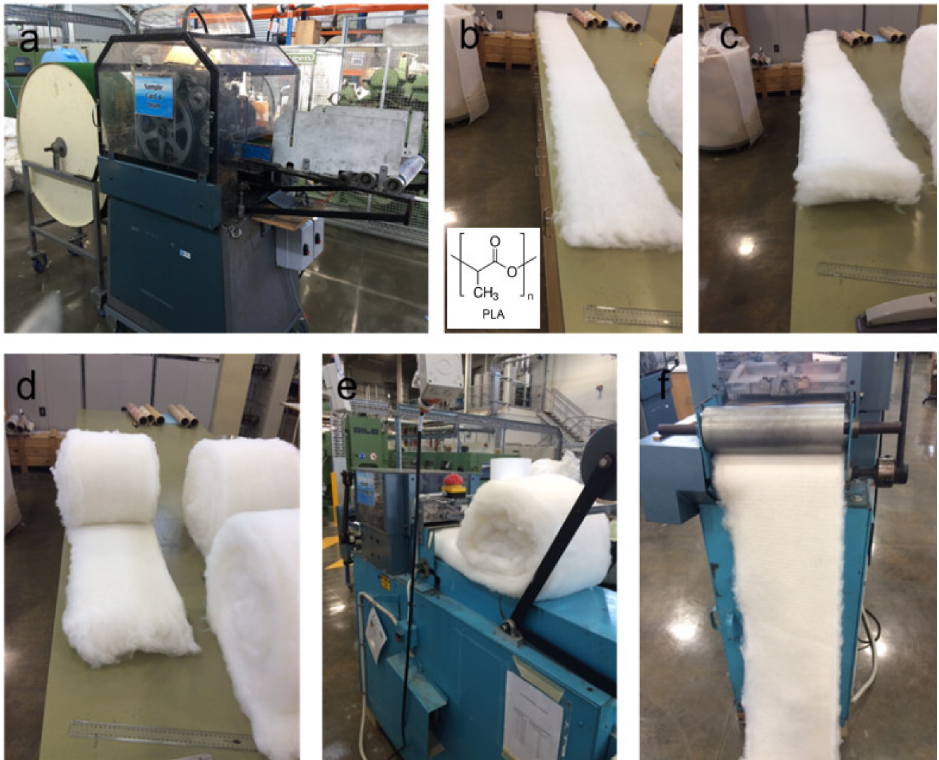
Figure 1. Processing nonwoven mats from cotton and PLA fibres. (a) Carding machine; (b) equivalent weight of cotton fibres and PLA fibres were hand blended firstly before putting through a carding machine twice for uniform mixing; (c,d) webs were then stacked into multiple layers; (e) 12 layers of webs went through needle punching machine at 30 punches/cm 2 on both sides; (f) nonwoven mats for the manufacture of composite panels.
