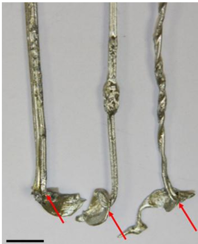
Fig. 3. Steel wires from tyres (arrow) recovered with a steel wire hook from the bottom of Leg B (bar = 10 mm).
