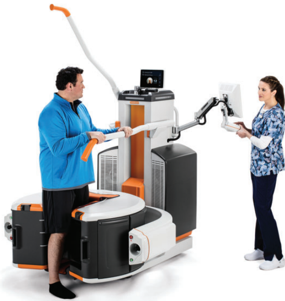
Figure 1. Acquisition of images in the prototype cone beam computed tomography scanner with a patient weightbearing on a flexed knee. Image reprinted with permission from Carestream Health.
