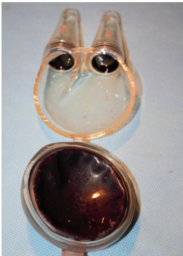
Figure 6. Deposits on the pump membrane.
