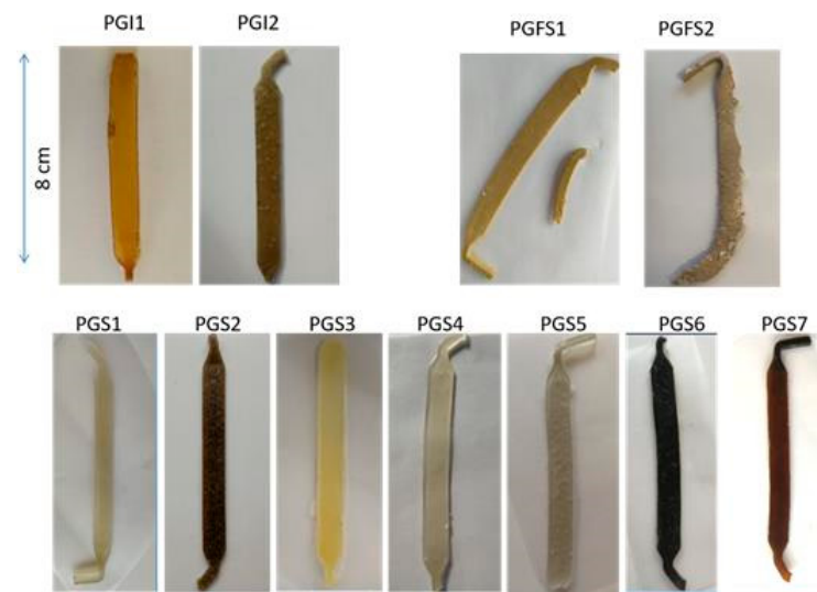
Figure 3. Photographs of elastomer sheets obtained by extrusion of their prepolymers when driven by the twin screws at a speed of 200 rpm and heated at 180 °C.
