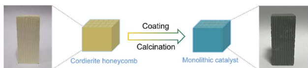
Fig. 1 Preparation route for the monolithic catalyst.
