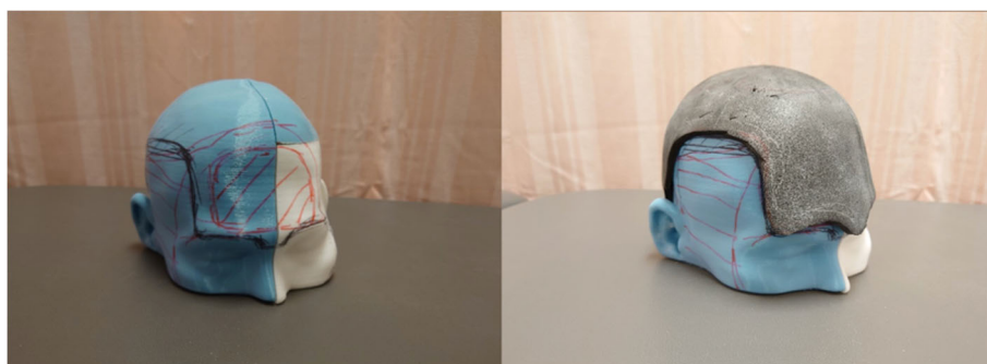
Fig. 5 (a) The 3D printed head model, with pressure-sensitive areas marked in red. The helmet border is marked in black (b) The head model fitted with 6 mm of Plastazote® foam
