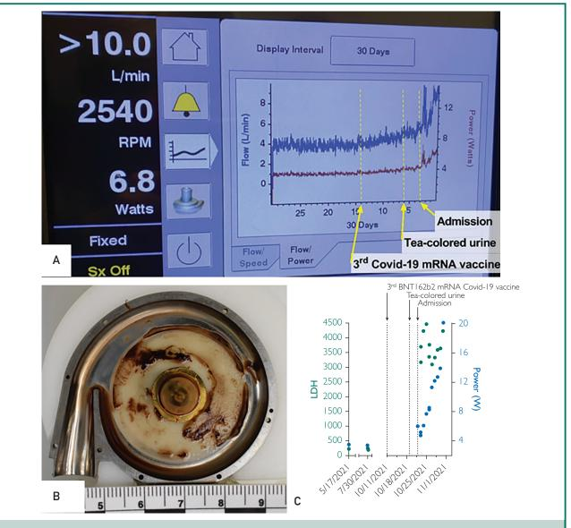
FIGURE. A, HeartWare power and flow waveforms during early hospitalization. Dates of Pfizer-BioNTech COVID-19 booster, symptoms, and admission are superimposed. B, Image from pathology report demonstrating evidence of thrombus within the HeartWare device. C, Timeline of HeartWare power and lactate dehydrogenase (LDH) in the context of thrombosis. Baseline values and dates of vaccination, symptoms, and admission are shown relative to biomarker trends.
