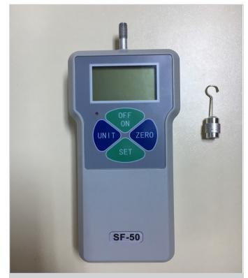
Figure 3. Digital Newton-meter that was used for measurements
