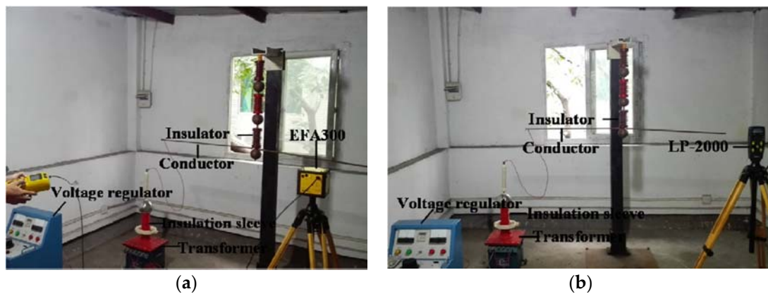
Figure 9. Experimental measurement (in the absence of a human body). (a) Measuring worksite of Narda EFA-300; (b) measuring worksite of Type LP-2000.
