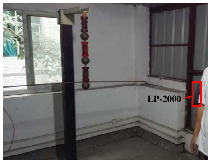
Figure 11. Measuring worksite of Type LP-2000 (in the case of an approaching human body).
