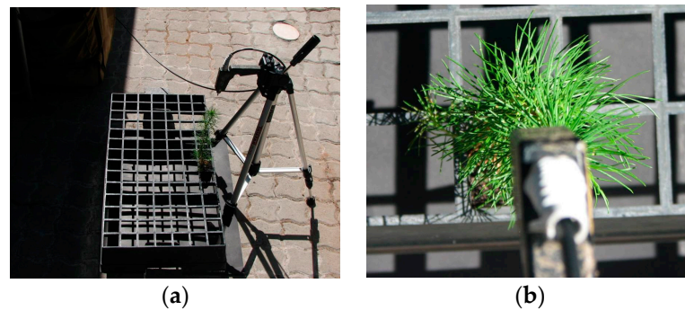
Figure 1. Experimental setup of the spectroradiometer used for spectral data collection (a) showing the orientation (nadir view) of the pistol relative to the seedling (b).
