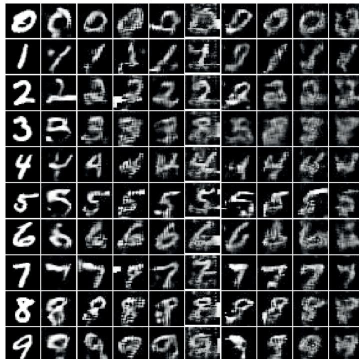
Figure 6. Examples of generated images when different compression rates were used for the vOICE encoding. Each row shows a gradual change of each generated MNIST digit image with the change in compression ratio. The left-most column contains unencoded MNIST digits; the second left-most column contains digits encoded by the vOICE, but not compressed; columns from third left-most to the right contain digits encoded with compression ratios from 10% to 80%, increased by 10%.
