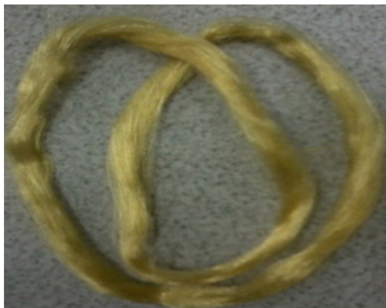
Figure 12. The photograph of the cellulose–chitosan composite fibres made by [152] using a binary ionic liquid system and the dry-wet spinning procedure. Reprinted from Carbohydrate Polymers , 88/1, Ma, Bomou, Zhang, Meng, He, Chunju, Sun, Junfen, New binary ionic liquid system for the preparation of chitosan/cellulose composite fibers, 347–351, Copyright (2012), with permission from Elsevier.
