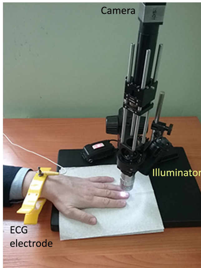
Figure 6. Video capillaroscopy setup for simultaneous recordings of ECG and microscopic video of capillaries.
