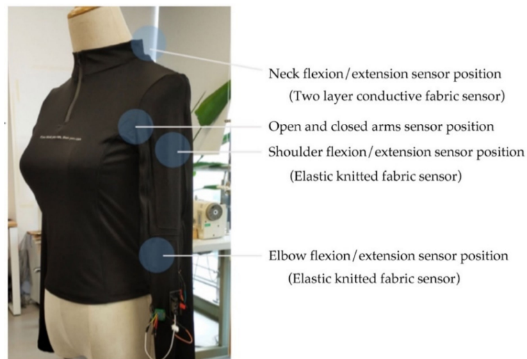
Figure 4. The female version of the E-MotionWear prototype and placement of the different sensors.
