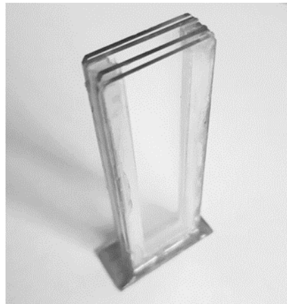
Figure 2. Phononic crystal sensor used for the experimental realizations.
