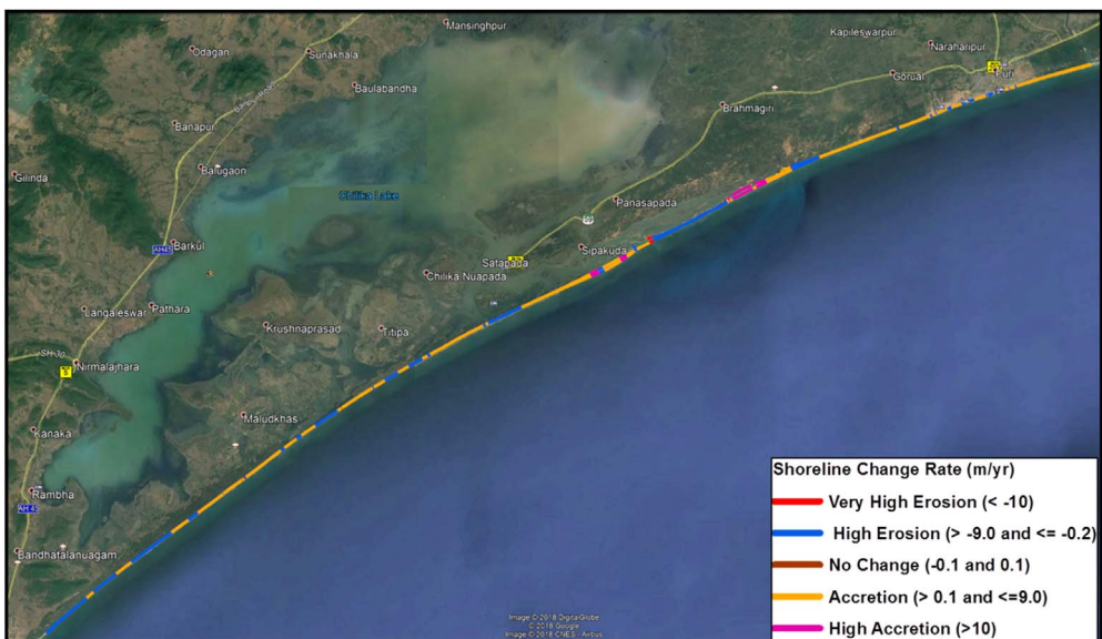
Fig. 3. Extracted shoreline was overlaid on Google earth image and classified into five classes based on EPR values.
