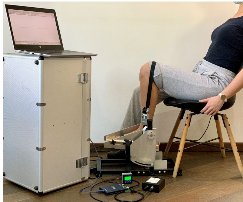
Figure 2. The system components used for ankle torque measurement and participant position on the chair; the measurement system components include: portable custom-made electronic dynamometer with an incorporated load cell, electronic inclinometer, a load cell amplifier, oscilloscope, connection wires and a PC.
