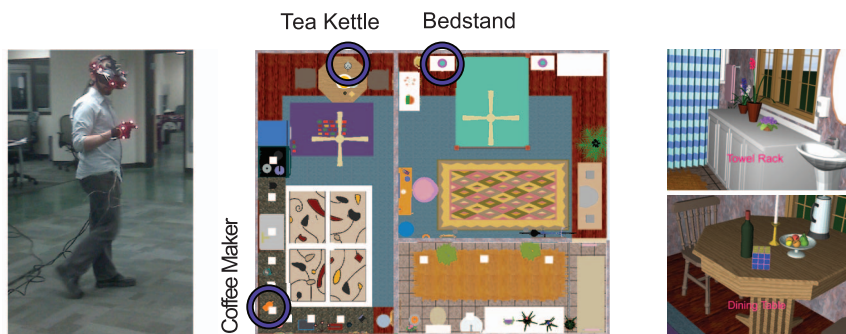
Figure 1. Subjects performed a visual search task within a virtual-reality three-room apartment. A. Subjects wore a V8 head mounted display (HMD) equipped with an ASL eye tracker, while the head and hand were tracked using the PhaseSpace motion tracking system. The subject touched virtual objects in the apartment using the gloved hand when they were located. B. Overhead view of the virtual apartment showing the three rooms: bathroom, bedroom, and kitchen. The 3 objects specified for repeated search are indicated by purple circles. C. Two example views, recorded while a human subject was exploring the apartment wearing the HMD. Targets were specified by words at the bottom of the screen (e.g., "Coffee Maker") and the subject had to locate and touch that object (e.g., the orange coffee maker). Gaze position, head orientation and location were recorded for later analysis.
