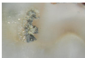
Figure 6. Cohesive failure—group B.
