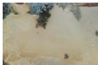
Figure 8. Mixed failure—group B.
