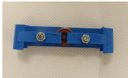
Figure 2. Modified stationary clamp for plastic cylinder stabilization.
