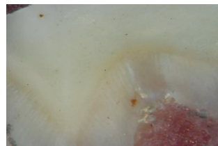
Figure 3. Adhesive failure—group A.
