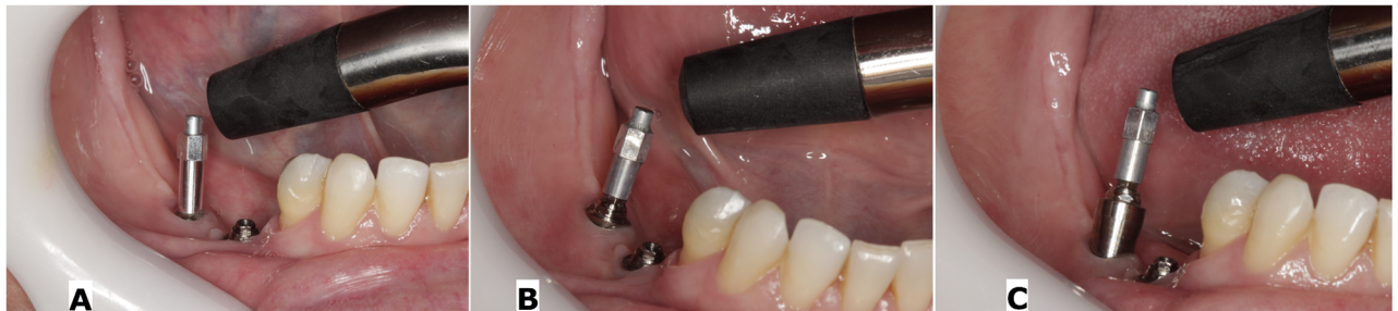
Fig 1. Resonance frequency analysis by Osstell. A) Implant platform B) 1mm microunit C) 5mm microunit.
