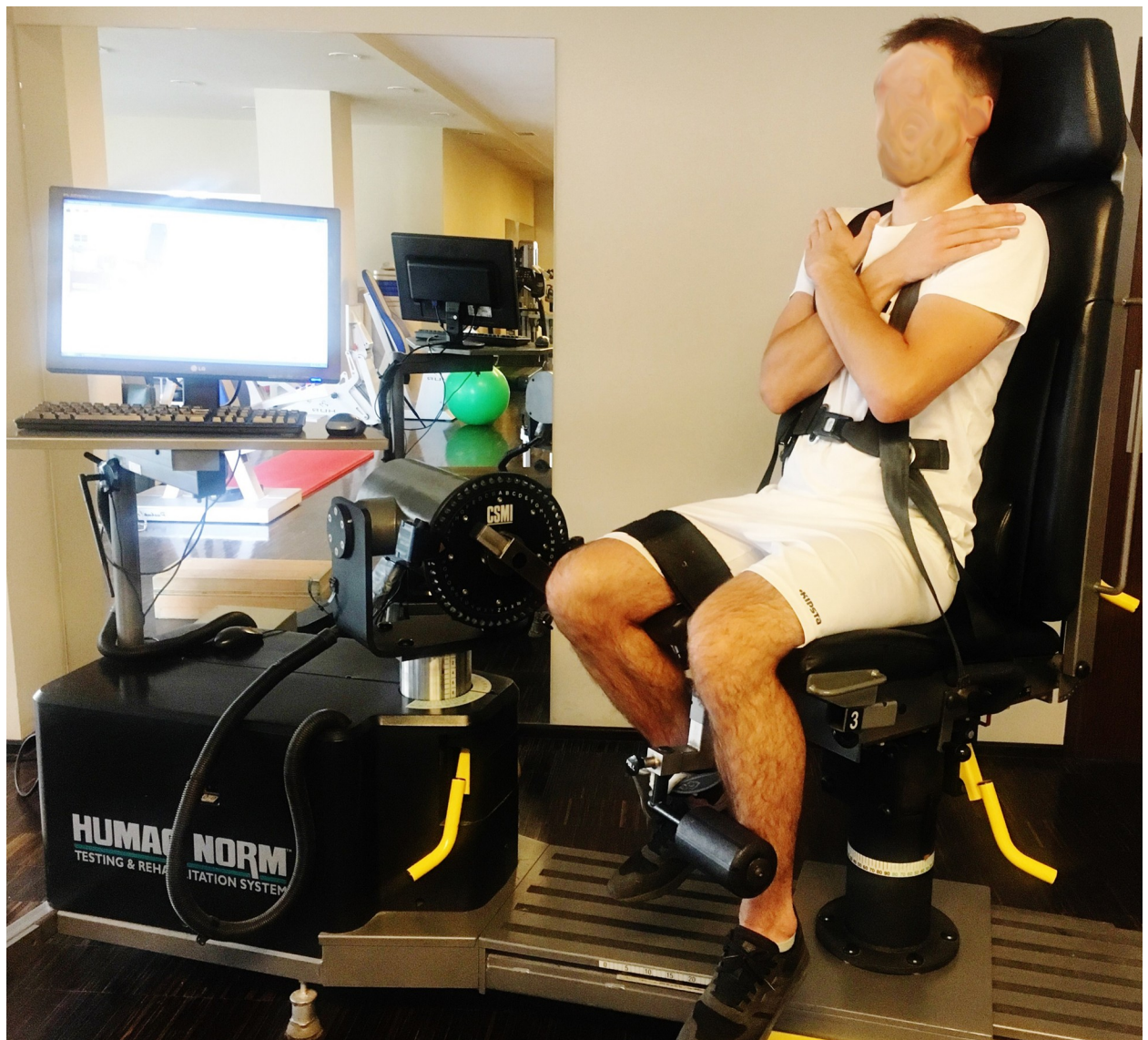
Fig 2. Maximal flexion of the examined limb as the final position for the knee flexor muscle PT measurements.
