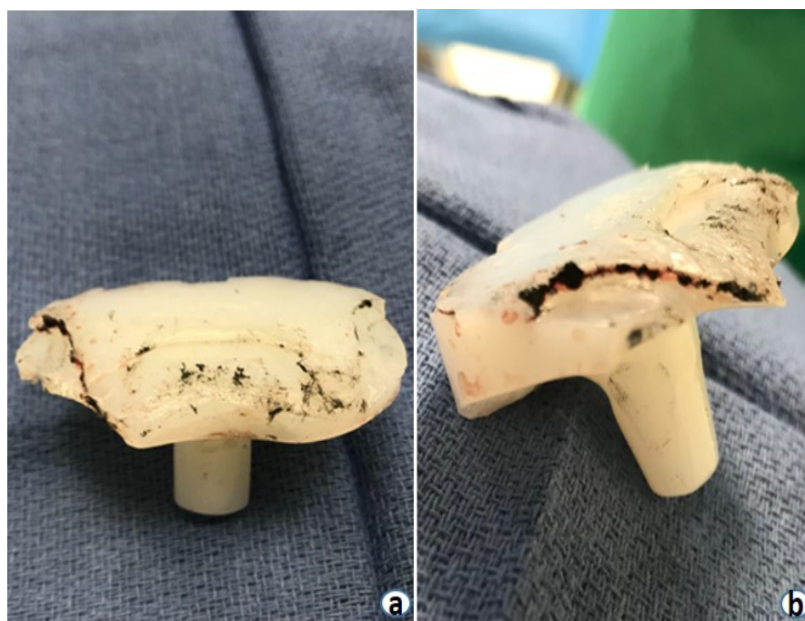
Figure 3: (a) Coronal view of polyethylene spacer demonstrating disintegration of the medial compartment. (b) Sagittal view of the polyethylene spacer further demonstrating disintegration of the medial compartment.
