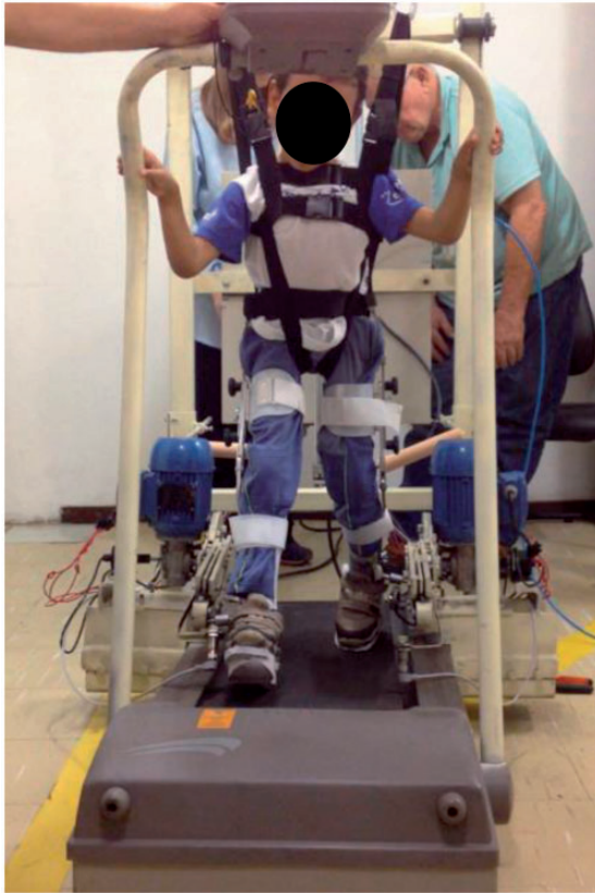
Figure 13. Prototype of the robotic orthosis attached to the treadmill.
