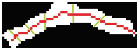
FIGURE 6: Binarized representation of a singular hypha (white pixel) with skeleton (red line) and perpendicular width evaluation along the exemplarily shown green lines.
