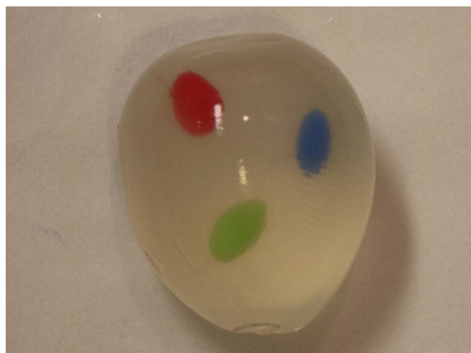
Fig. 2. A prostate phantom with three focal lesions. A total of 0.5 mL of warm agar solutions stained with red, blue, and green ink was injected using a 1 mL syringe to simulate a focal lesion in the prostate phantom. Each lesion is located at base, midgland and apex of the prostate phantom.
