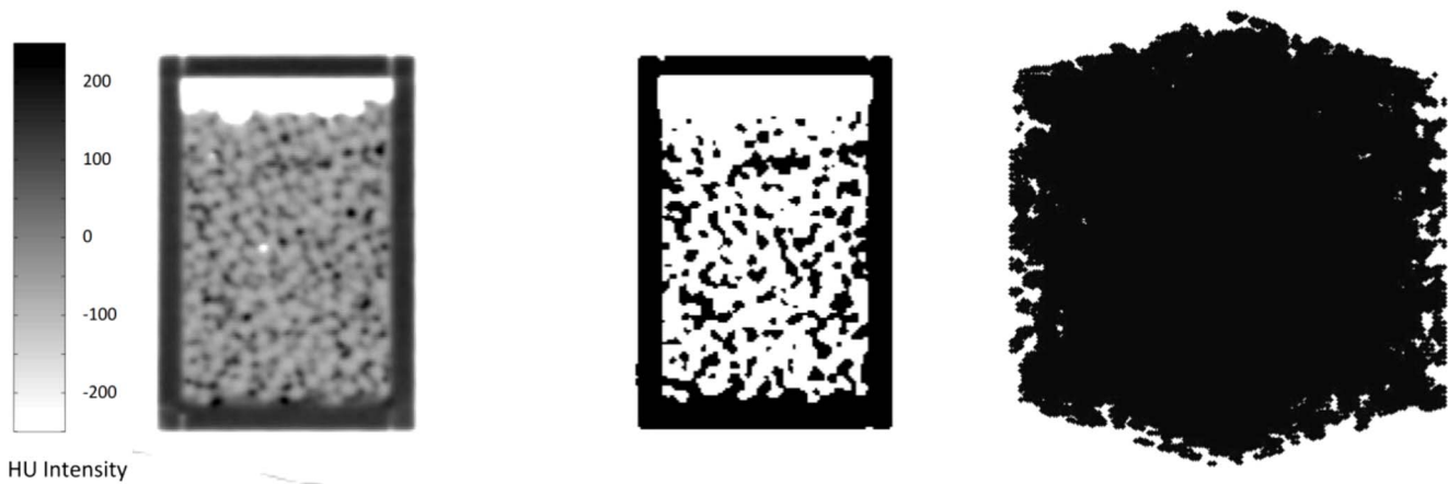
Figure 3. Sample original (A) and masked (B) CT slice and an example of fixed particles arrangement (C). doi:10.1371/journal.pone.0067958.g003
