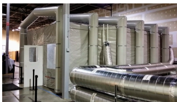
Figure 5. Mobile environmental exposure chamber (mEEC) used for the controlled clinical study.
