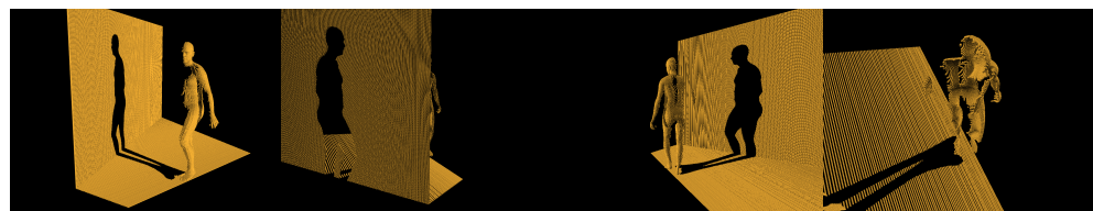
Figure 3. An example of neural network input that is created rendered depth frame converted to pointclouds with the help of camera intrinsic matrix K .
